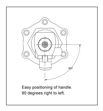
Saftey Handle helps to prevent accidents while changing rivet snaps or while being carried with the air hose still connected.
